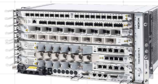
NOKIA ISAM FX-4 Optical Line Terminal (OLT) FTTH- und Smart Meter-Rollouts
